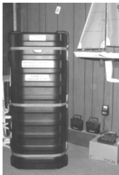
inforced with cross members to react to loads from the boat egg crate foam protectors. The design was very tight to fit the two complete mast/sail assemblies in the sail box.
