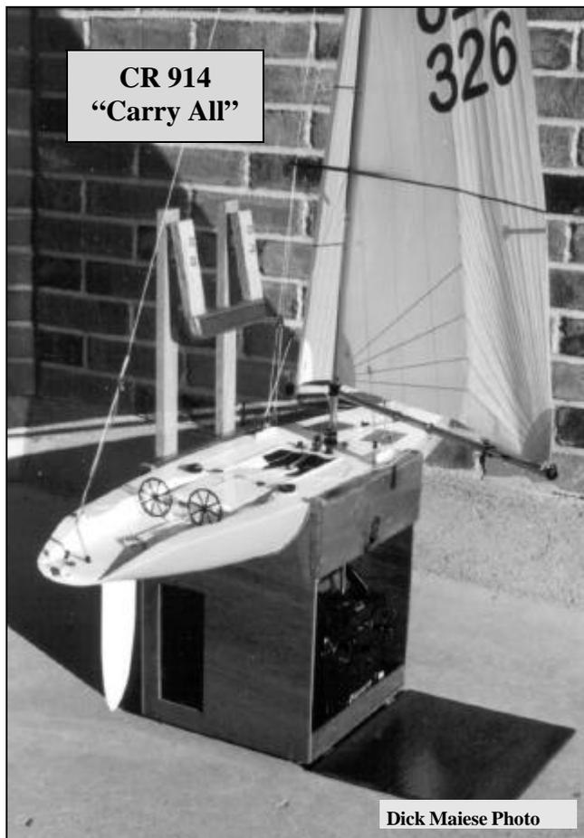
form for setting up and tuning the rig with equipment close at hand. The unit resists blowing over even in heavy air especially if the bow is turned into the wind. It weighs less than 4 pounds.
