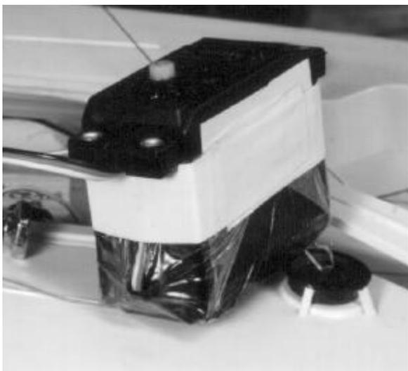
easy to do and should be quite effective. It seals all the leaks except the one at the output shaft on the top. Apply Vaseline liberally at the output shaft.
