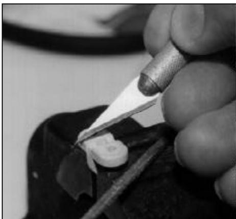
Groove the eyelet to recess the line
