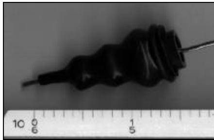
mechanically rugged. It is best to have the female portion on the battery lead. There is always the chance that the exposed pins of the male portion could be shorted by contact with something conductive.
